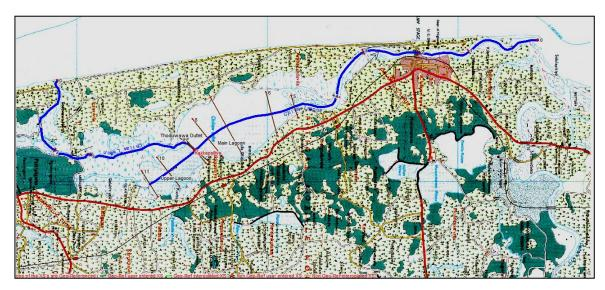
13. The Model test was carried out to verify how the flood inflow canbe absorbed by the lagoon and to see whether a storm event with two-year return period can effectively flush out the lagoon and its outlets. Freshwater inflow due to the storm event with a two-year return period is about one million cubic meters.
